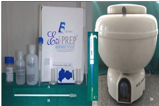
Fig. 1: Armamentarium for CLBC. A) Eziprep LBC Kit B) Cytobrush C) Micropipette D) Centrifuge
